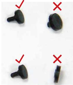
POSSIBLE CAUSE: Ball Detents are damaged.
