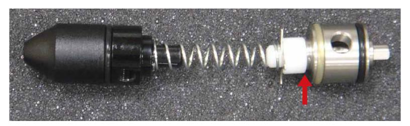
POSSIBLE CAUSE: Damaged Valve.
