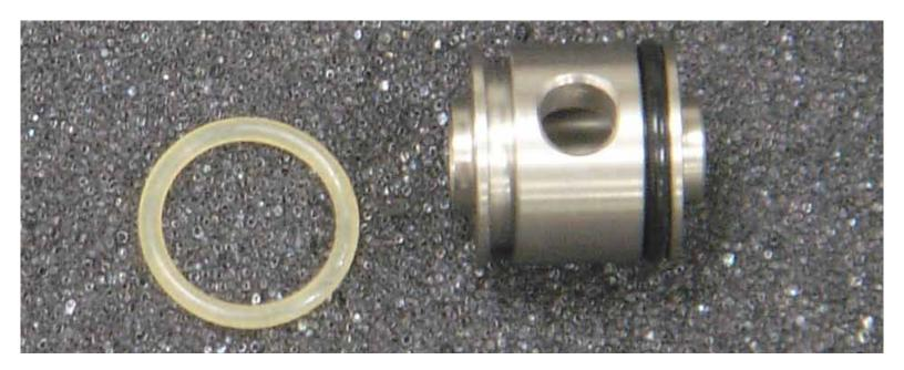
POSSIBLE CAUSE: Front Valve O-Ring (R012) is damaged.
