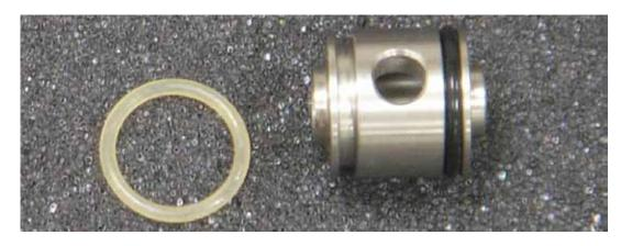
POSSIBLE CAUSE: Front Valve O-Ring (R012) is damaged.
