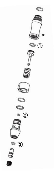
① POSSIBLE CAUSE: Regulator Piston O-Ring is damaged.
