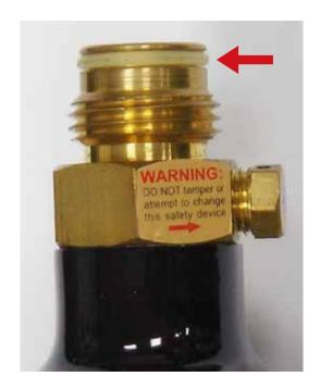
POSSIBLE CAUSE: O-Ring on the air tank is damaged.
