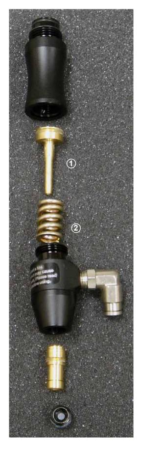
POSSIBLE CAUSE: Poorly maintained Inline Regulator.
