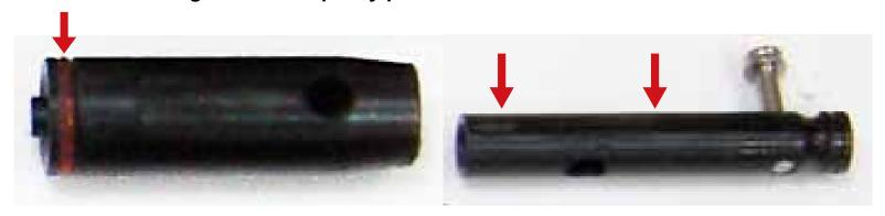
**SOLUTION:** Needs lubrication on striker and bolt.
