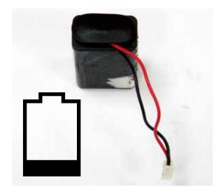
POSSIBLE CAUSE: Battery has insufficient power.
