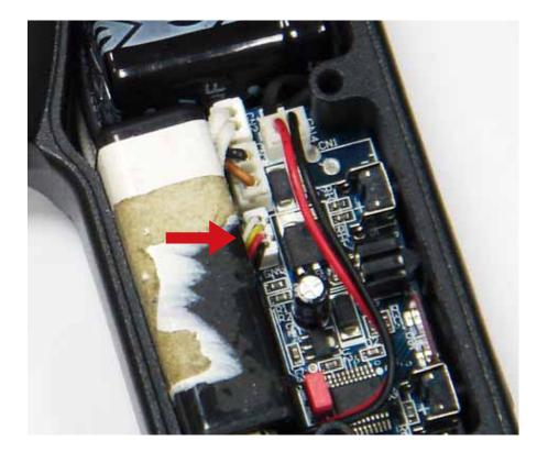
POSSIBLE CAUSE: Damaged eye sensor wire.
