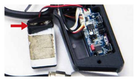
**POSSIBLE CAUSE:** The battery terminals did not connect to battery harness.
