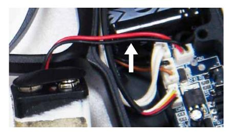
POSSIBLE CAUSE: Battery harness is damaged.
