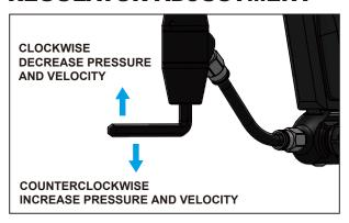
To increase the input pressure, use the allen wrench to turn the RockSteady Seat (RSS2) counterclockwise.
