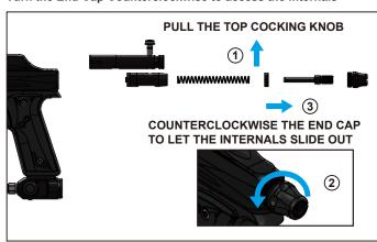
WARNING: Never remove the internals of the marker while the tank is attached to the marker. Always remove the loader, the air tank, and all paintballs from the marker before disassembly.
