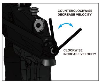
To increase your velocity FPS (Feet Per Second), use the allen wrench to turn the Velocity Adjuster (VA01) clockwise.
