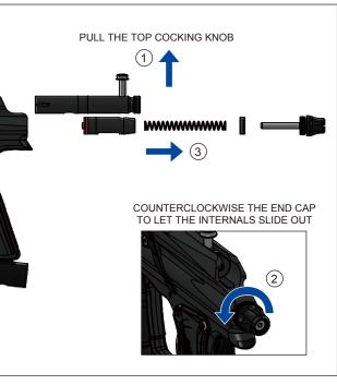
WARNING: Never remove the internals of the marker while the air tank is attached with the marker. Always remove all paintballs, loader and air tank before disassembling the marker.
