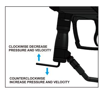
Adjusting the regulator will change the amount of pressure entering the marker. Regulators are preset for optimum performance from the factory and most adjustments should be made through the rear velocity adjuster.
